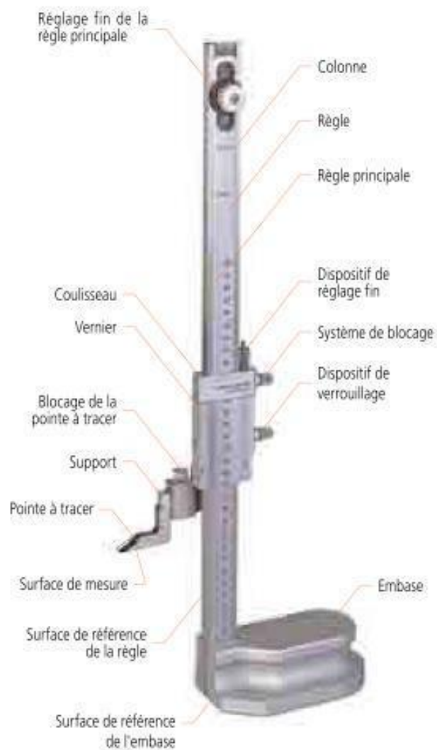
Fig I.6 – Trusquin a vernier.
